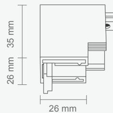
**CONECTOR CODO (EXTERNO) AC5512N / AC5548N**
