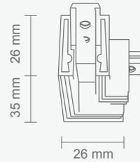
**CONECTOR CODO (INTERNO) AC5511N / AC5547N**
